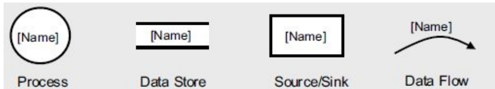
Figure 6-10 Important modeling elements of data flow diagrams according to DeMarco
